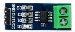
The 5A range Current Sensor Module ACS712 consists of a precise, low-offset, linear Hall circuit with a copper conduction path located near the surface of the die. Applied current flowing through this copper conduction path generates a magnetic field in which the Hall IC converts into a proportional voltage.
