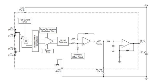
• The ACS712 Module uses the famous ACS712 IC **to** measure current using the Hall Effect principle. The module gets its name from the IC (ACS712) used in the module, so for you final products use the IC directly instead of the module.
